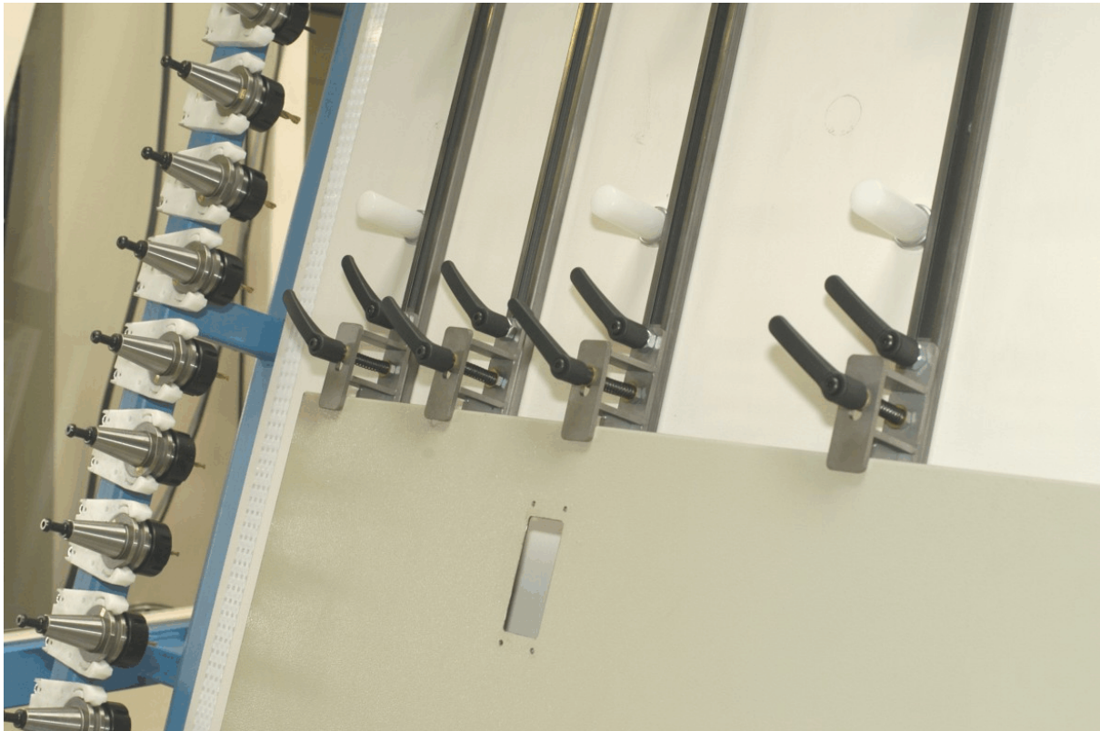
Picture.: Tool magazine with upper front side mechanical quick action clamps.
