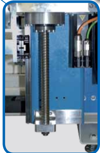
Chip-resistant positioning techniques with ball screws and linear guides on all axes
