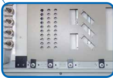
Pneumatic frontside part fixture 7 pneumatic muscles at the base of the machine's frame hold flat workpieces in place at the push of a button. The muscles can be switched off individually to avoid blocking areas in the clamping range. The coating under the fixing points remains undamaged.
